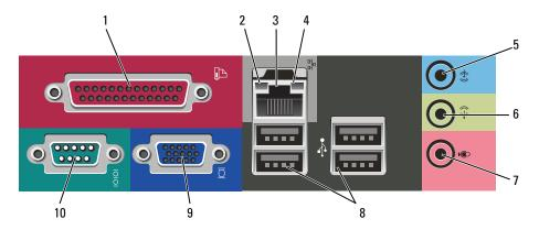
1 parallel connector Connect a parallel device, such as a printer, to the parallel connector. If you have a USB printer, plug it into a USB connector.
